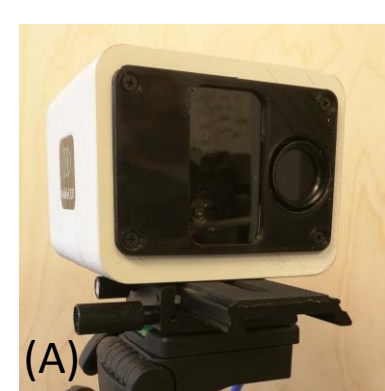
Fig. 2: (A) Optical head of multi-spectral device, with camera on right and LED board on left. (B) Entire setup, showing optical head mounted on tripod and coupled to a tablet.
